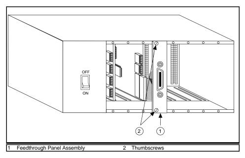
Figure 2-2. Completed Installation for the STD-GPIB
